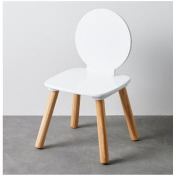
**Defect:** The three screws used to attach the legs to the base of the chair may be too short, and if a child rocks on it, leans on it at an angle, or climbs on it, the chair may break.
