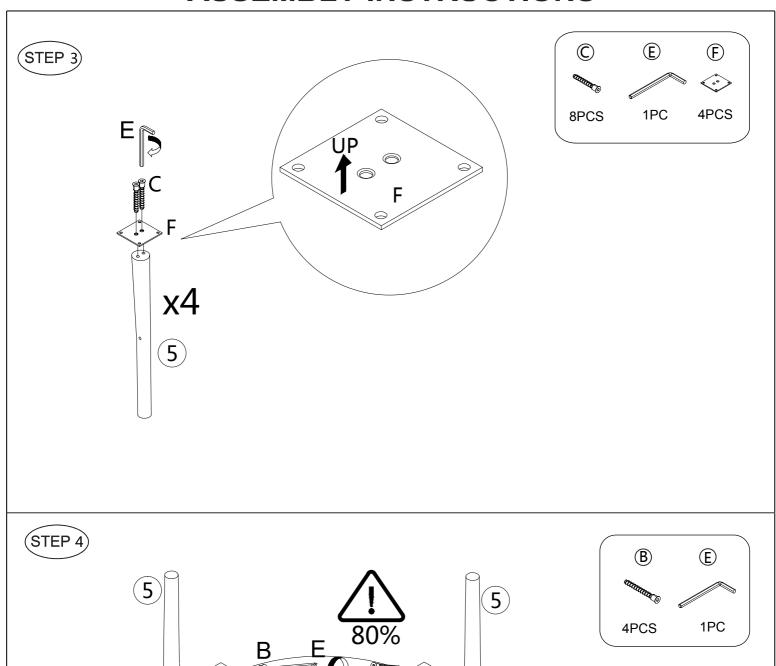
Please do not tighten all screws in this step until both step 4 and step 5 screws are well align.
